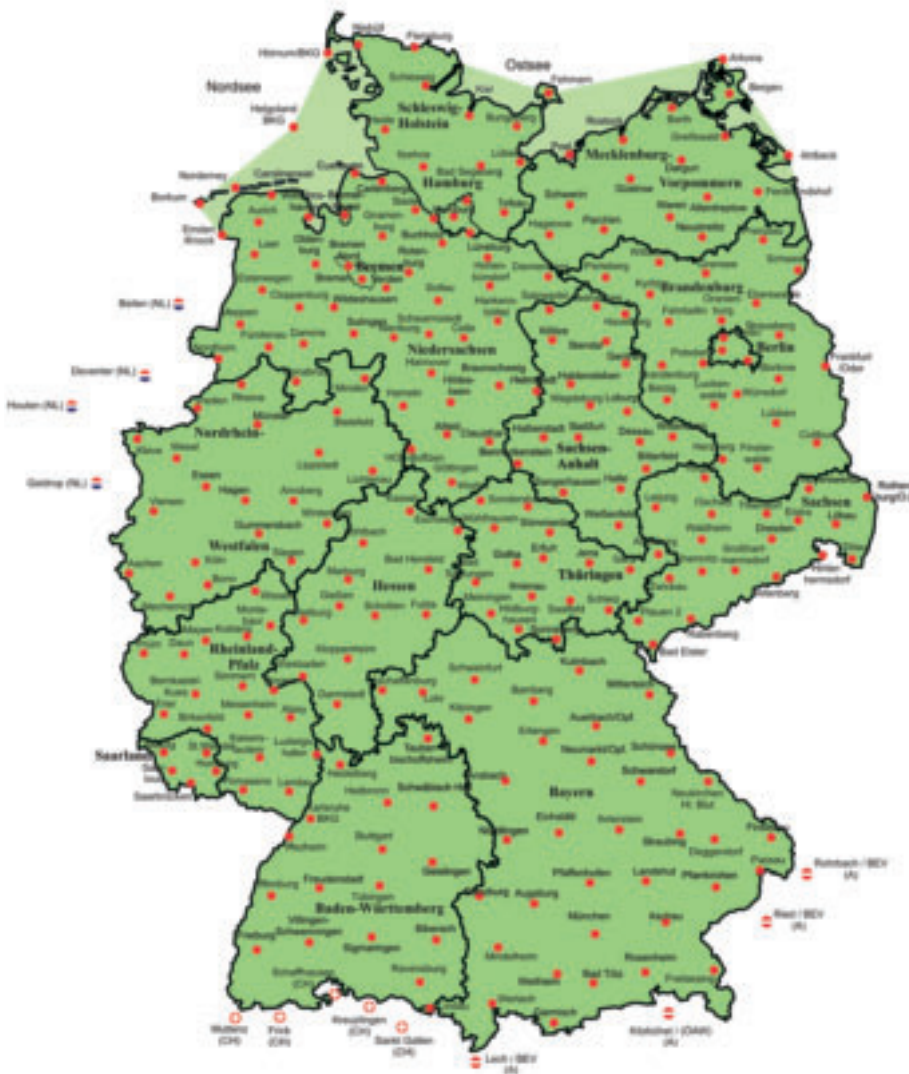
Figure 1. SAPOS reference stations with location (real-time networking).
